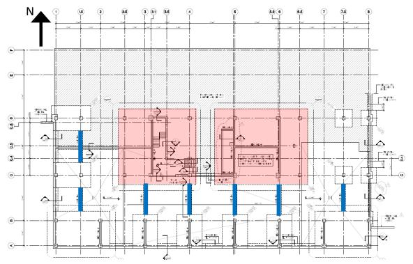
Figure 2: Foundation Plan (Level PO) Showing 48" Thick Mat Foundations Shaded in Red (Source: Cagley & Assoc. Drawing S-200)
